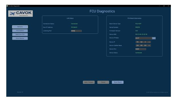
The network page shows the current status of the LAN connection and allows you to change the LAN settings of the FCU board. As soon as the device is connected and recognized, the device status changes to connected and all current settings are displayed. All gray boxes can be changed by the user.
