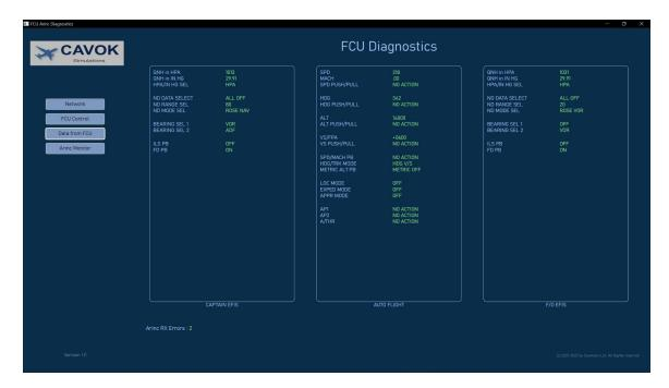
This page shows all decoded data that is received from the FCU via Arinc messages and electric signals. It allows you to quickly test the function of all buttons, switches and rotary encoders of the FCU.
