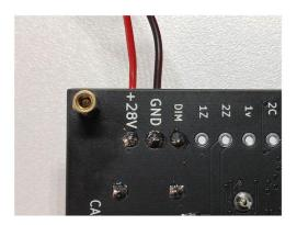
Figure 5 - Wiring of the Power supply
