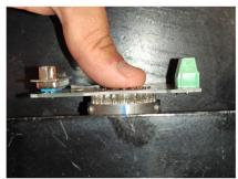
4. Photo shows adapter in fully inserted position
