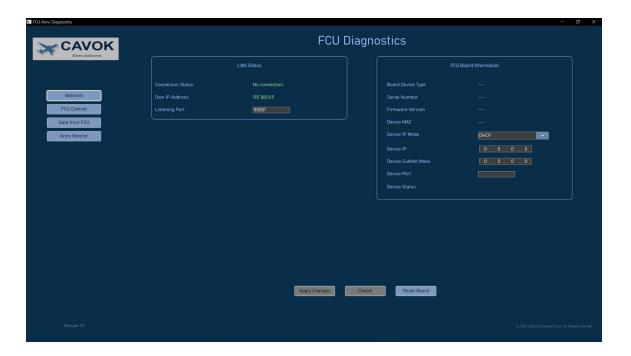
The software will now try to find and establish communication with the FCU board via the LAN network and the UDP port shown in the field "Listening Port". The default port for the FCU board is 50001.
