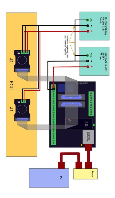
Figure 2 - Overview of the board connections
