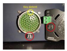
1. Check that connector and adapter type match
