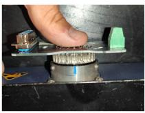
3. Apply pressure to the center and parallel to FCU
