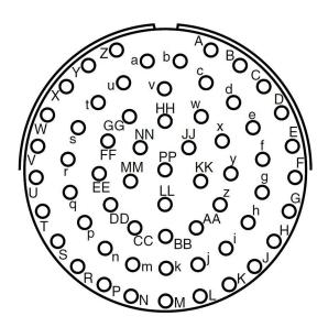
The male MIL-DTL connectors also have the letter labels printed on the connectors close to their pins similar as shown in the diagram above.
