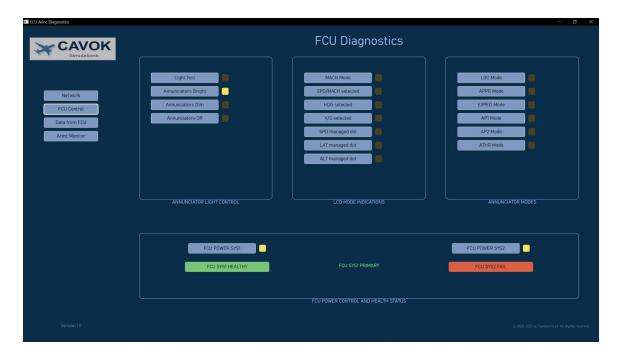
The FCU Control page lets you switch the FCU on or off for testing and send commands to the FCU to test all major functions. A yellow square beside the buttons indicates if a function is currently active.
