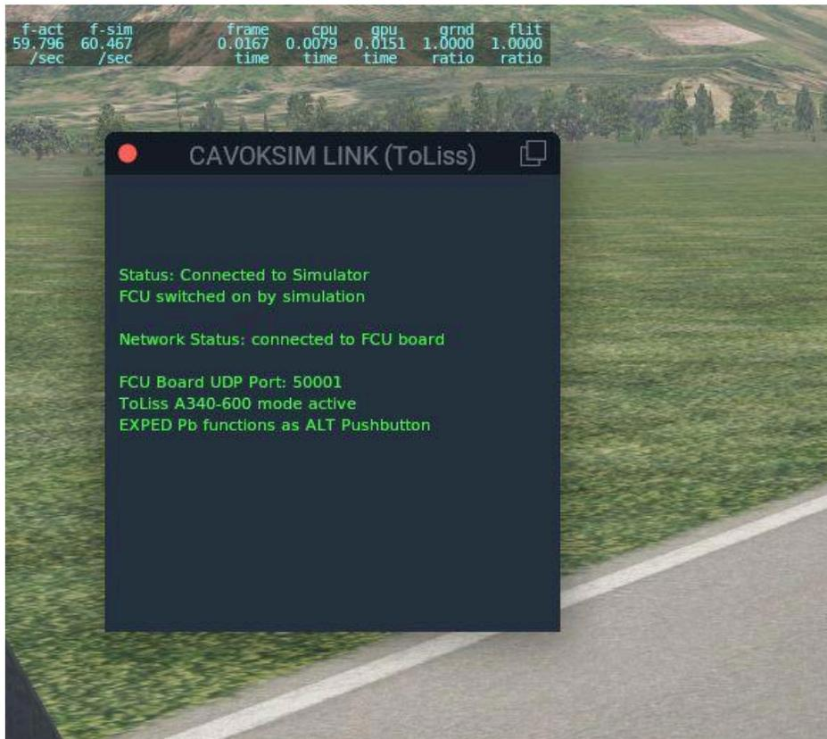
The status window provides various status information. In normal operation, all text should be in green. Yellow text indicates warnings and red text indicates failures.
