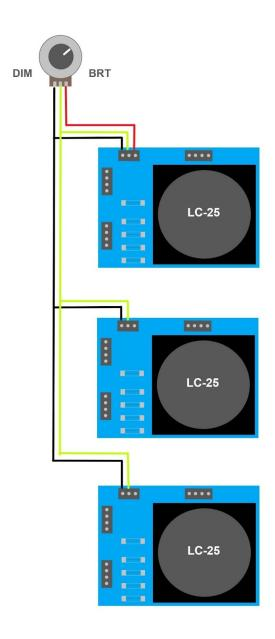
Figure 2- Connecting the same potentiometer to several controllers
