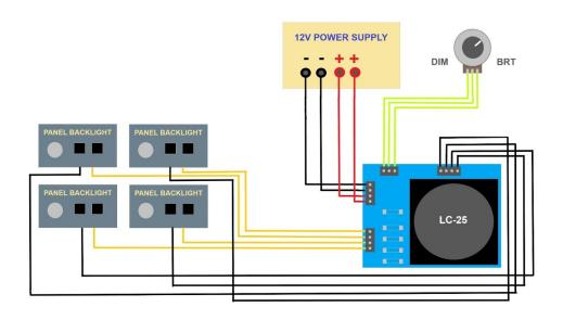
Figure 1- Wiring example for a single controller
